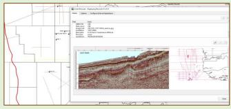
18 cross-sections linked to a raster image which pops-up when clicking on the well (using e-vis event tool in QGIS or html popup tool in ArcGIS).
